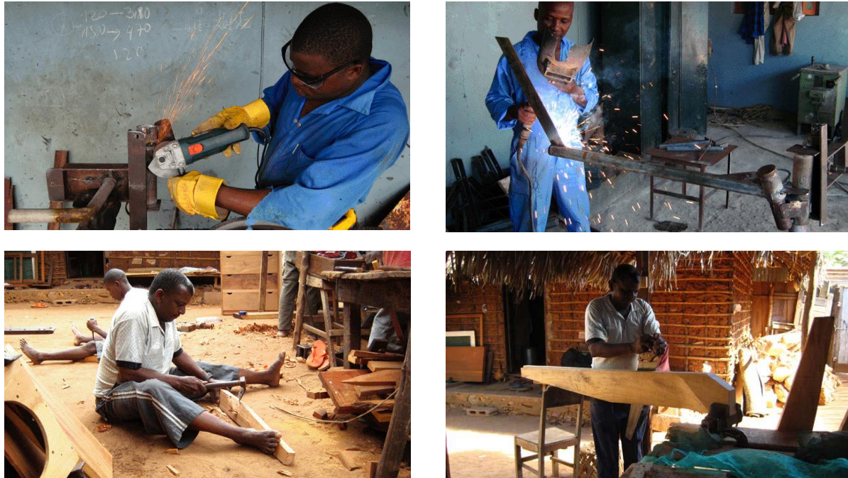
FIGURE 4: MANUFACTURE OF A SWT USING SIMPLE TOOLS AND TECHNIQUES IN MOZAMBIQUE. PHOTO COURTESY OF THE CLEAN ENERGY INITIATIVE.
