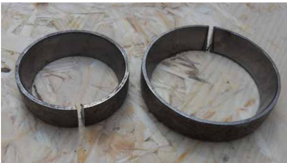
Fig. 39: Cut the shell with an angle grinder
