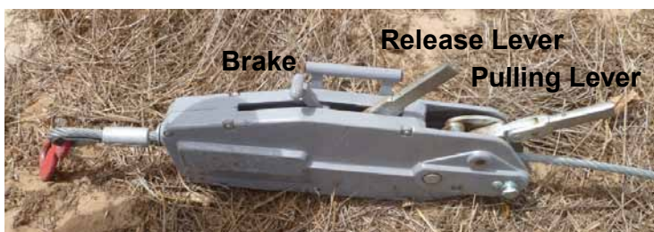
Fig. 10: Wire pulling grip hoist
