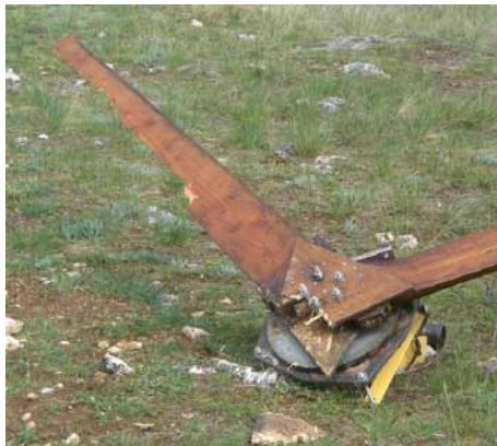
Fig. 64: Loss of balancing weight
