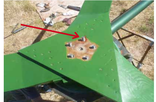
Fig. 17: Mark on a threaded rod and triangle
