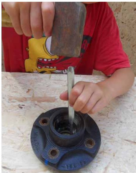
Fig. 38: Take out the outer shell
