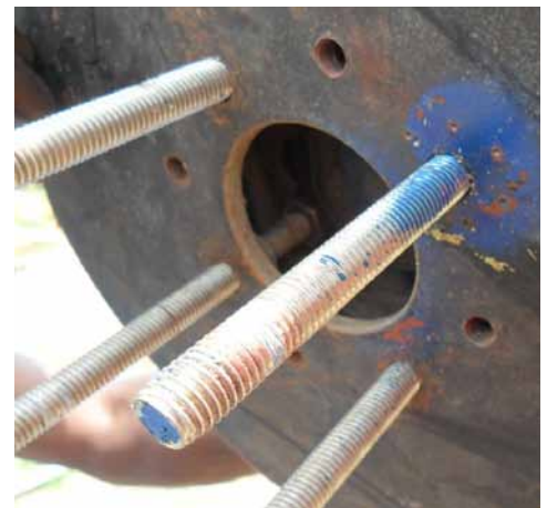
Fig. 29: Index threaded rod and hole
