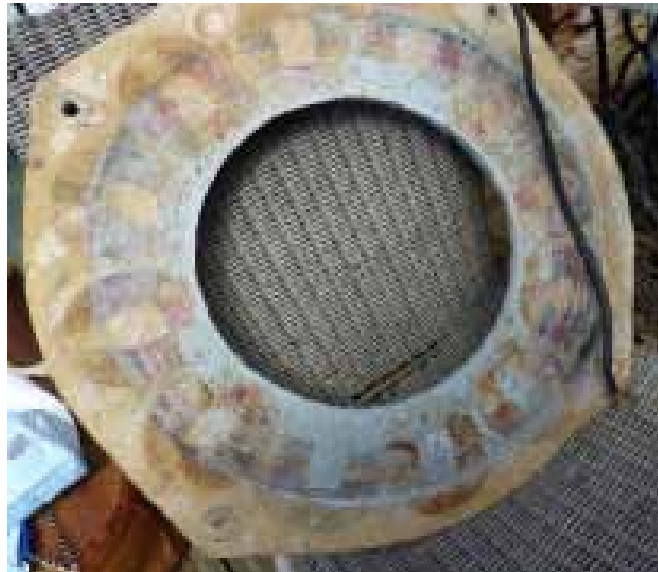
Fig. 31: Friction on the stator
