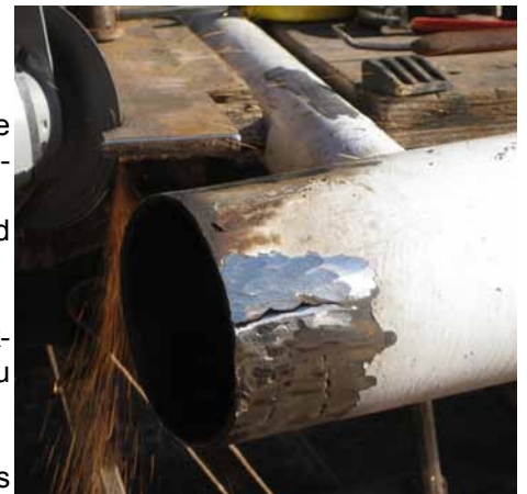
Fig. 44: Crack in the tail pipe
