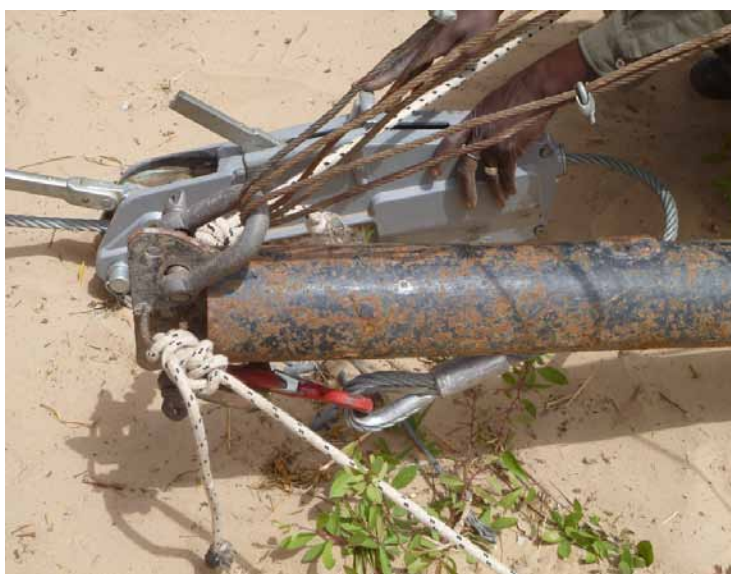
Fig. 11: Extremity of the gin pole with the grip hoist
