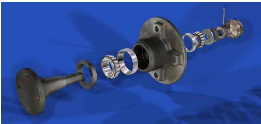
Fig. 36: Exploded view of a whole bearing
