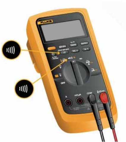
Fig. 54: Multimeter on continuity position
