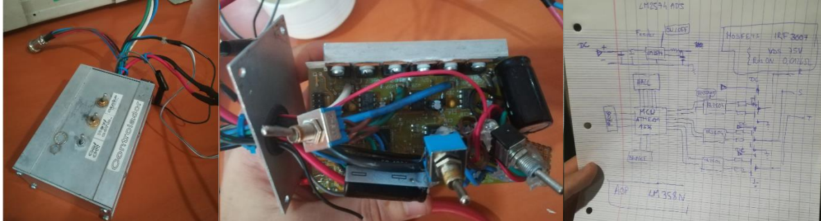
Figure 18 Pictures illustrating the reverse engineering procedure. The Argentinian proprietary converter in order to understand its behavior.
