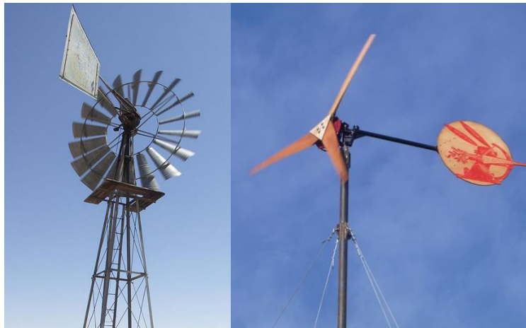
Figure 1 Illustration of a mechanical coupled wind water pump (on the left) and an electrical coupled one (on the right)
